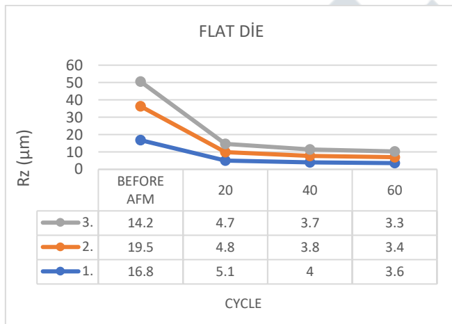
Fig. 11. Rz values of flat die before and after AFM
